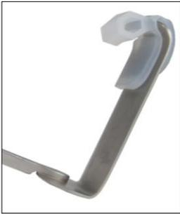
FlexGuard Retractor Blade Cushion. FlexGuard is a sterile, disposable accessory for standard surgical retractor blades (manual or self-retaining) designed to increase patient safety. FlexGuard is made from surgical grade Silicone having an open hexagonal cushion which serves as a shock absorber with two wings and has an adhesive strip on the back.
